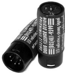
On the last instrument will you need to place a terminator. This is simply a male 3-pin or 5-pin plug that has a 120Ω resistor soldered between pins #2 and #3. When you use the end cap on the last DMX device you are closing the DMX circuit. This keeps the signal strong within the DMX line. I know many electricians who keep spare terminators in their pockets when setting up a show. (You always seem to need one when you are on top of a ladder or walking on a hung truss over a stage.)
