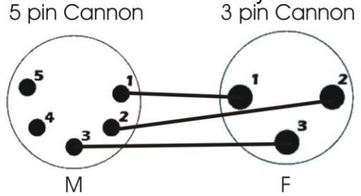
The temptation after that would be to use standard microphone cables because they use 3-pin XLRs at both ends. But if you use microphone cables you will be placing your DMX signal at risk because they do not have the electrical characteristics that DMX requires. DMX needs a cable that has an impedance of 120Ω and a capacitance of no more than 40 pF per meter. Essentially, this means that you need cable that uses a larger gauge than what is commonly used in microphone cables.
